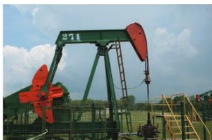
▲ Figure 7.1.1 A “nodding donkey” used in oil extraction
